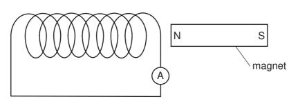
How could the ammeter reading be increased?
