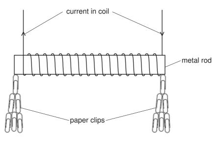
Each rod is used to pick up as many paper clips as possible. The current is then switched off.
