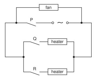
The fan has a power rating of 0.1 kW and the heaters each have a rating of 0.4 kW. The cost of electricity is 8 cents/kW h.
